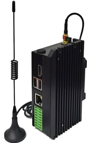
The Elastel EG410 is an industrial IoT Edge Gateway designed for IoT applications. Powered by Raspberry Pi CM4 with rugged, fanless design, it's perfectly execute Data Acquisition, Edge Analyzing, and communicate with cloud service via 4G LTE/3G/2G/ CAT M1(eMTC) and NB-IoT cellular network, Dual-band 2.4GHz/5GHz Wi-Fi, Gigabit Ethernet diverse network connectivity.
