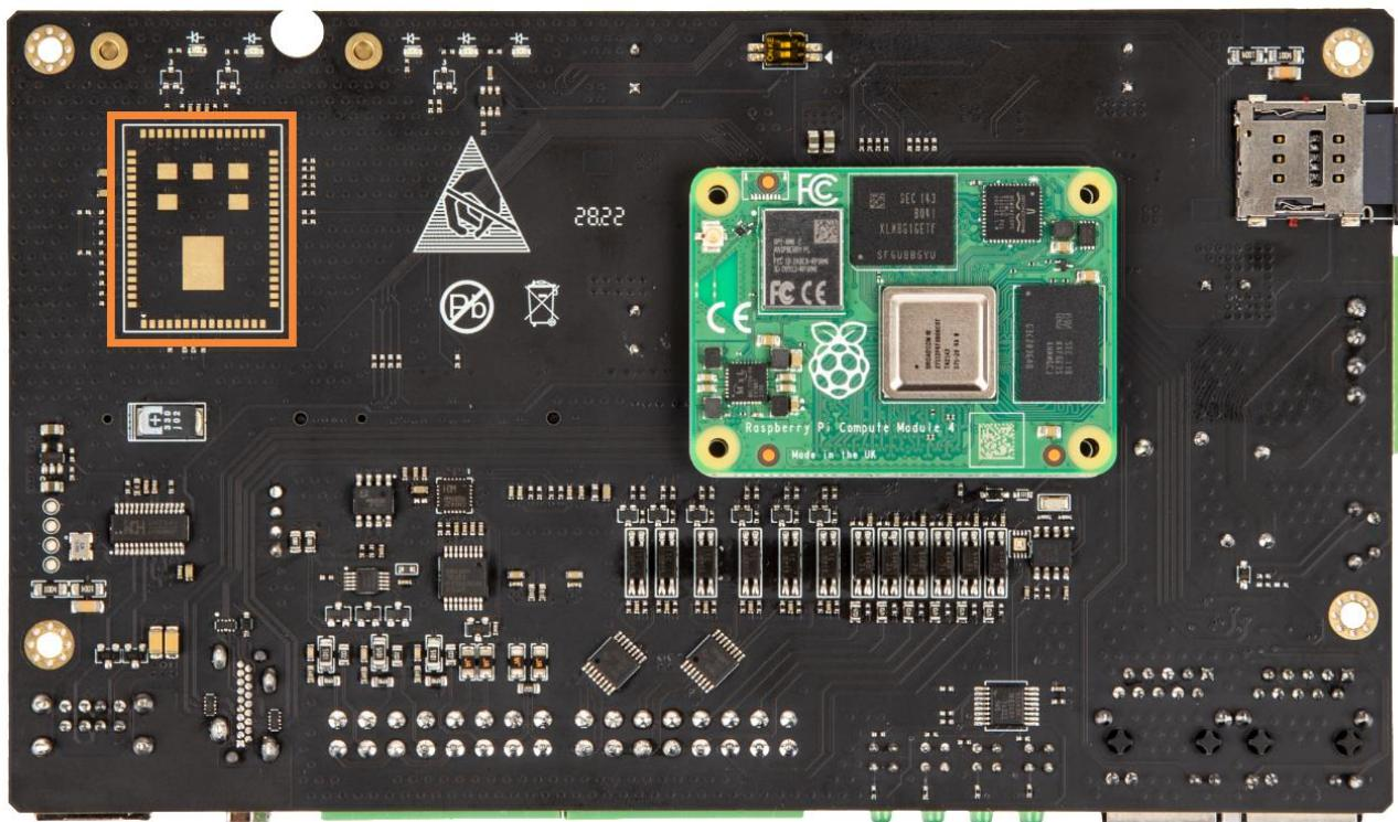
EG500 IoT gateway support 802.11ah WiFi (also named WiFi HaLow) network powered by SX-NEWAH module from SilexTechnology, the first industrial IEEE 802.11ah Wi-Fi module that operates in the Sub 1GHz band.
