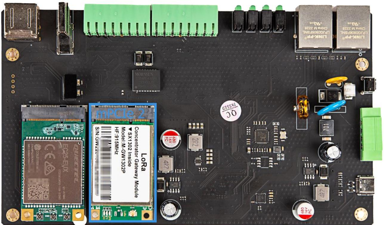
EG500 reserved another mini-PCIe socket for LoRaWAN module which develop from Semtech SX1301, SX1302 solution. Users are allowed to install a LoRaWAN module into mini-PCIe socket 2 as drawing blue area add-on module position, only one M2x5 screw is needed.
