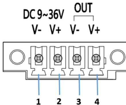
EG500 right side panel provide a 4-pin terminal block connector for Power input and a bridge connection for power output. The definition of PIN 1 “V-” as GND, PIN 2 “V+” for 9V~36V DC input. While PIN 3 & PIN 4 is a parallel power from PIN 1 & PIN 2, which considering designed for slave devices power supply.
