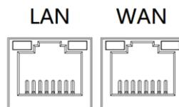
EG500 provide two Gigabit Ethernet ports, the one came out from Raspberry Pi CM4 is pre-defined as WAN port which supports up to 1Gbps link speeds over standard shielded CAT5e or CAT6 cables. The connector is the industry standard RJ45 connector.
