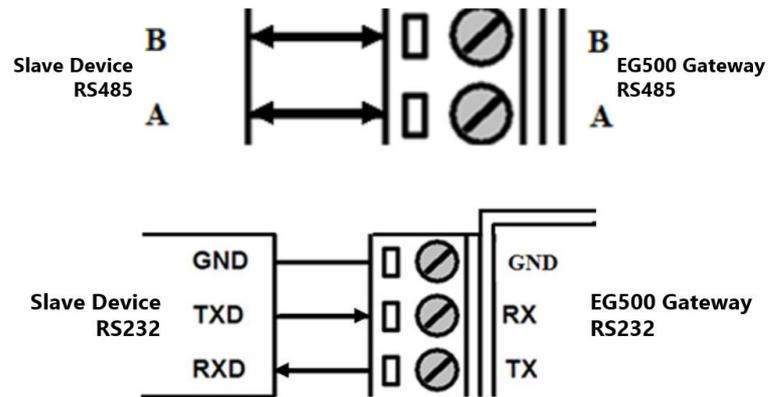
EG500 provide isolated serial COM ports, 1x RS485 and 1xRS232, the PIN B1\_15 defined RS485\_A (difference line high), PIN B1\_13 defined RS485\_B (difference line low).
