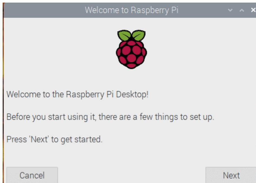
The Raspbian desktop version provide GUI desktop for operation. You will need a HDMI type screen, USB keyboard and mouse. Connect your screen to EG500 HDMI port, USB keyboard and mouse to EG500 USB ports. Now power on the EG500, you will be greeted with the Raspbian welcome screen, configure each steps following the setup wizard, and the EG500 is ready for use.
