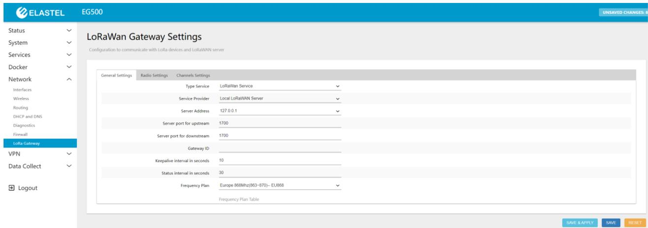
EG500 support add a LoRaWAN module powered by SX1301/1302 solution, and the webUI provide corresponding configuration to communicate with LoRa devices and LoRaWAN server.
