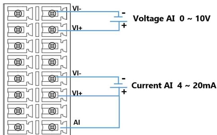
EG500 provide 3x Analog input ports with two types of analog signal, 4-20mA current input, or 0-10VDC voltage input.
