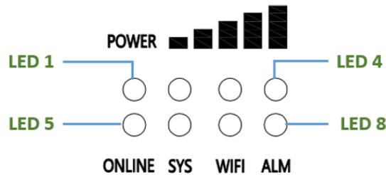
EG500 extend 8 LED indicators for apparent status indication as printed label shown, LED1 is defined as Power indicator which on once power on.
