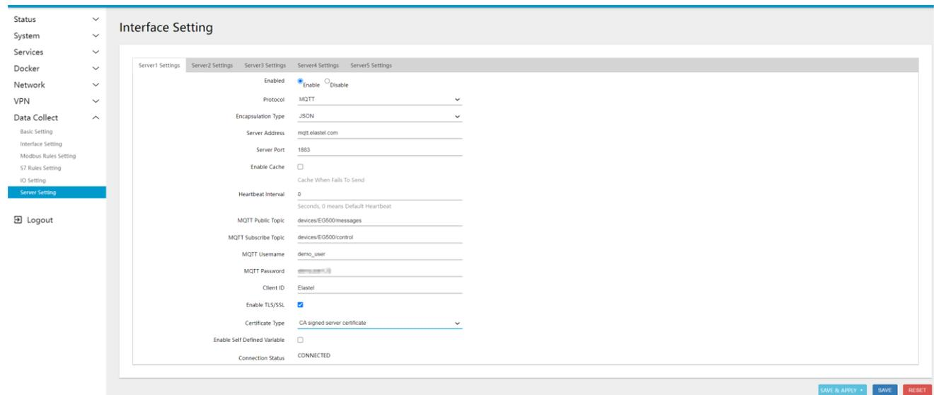
Server setting menu allows user set the data center address up to 5 servers with individual protocols. The EG500 support TCP, TCP Server, UDP, HTTP, MQTT, and Modbus TCP protocols for communication.
