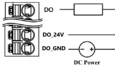
EG500 provide 6x DO to control the external slave devices. With an overvoltage protection circuit that DO 24V wiring, it could filter the overvoltage to avoid destroying device itself.
