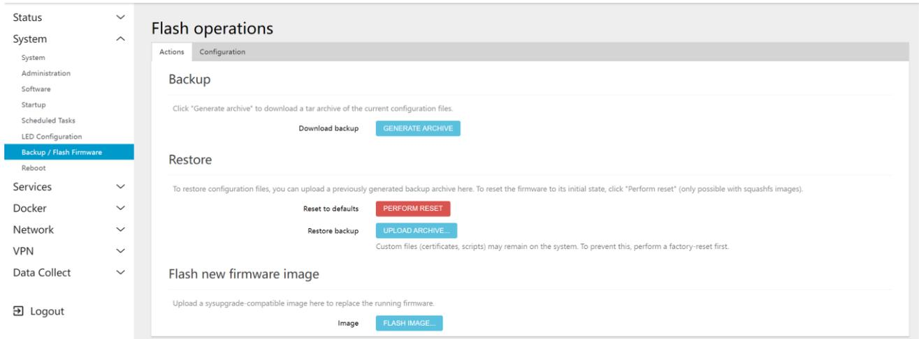
This page provides the operation of current configuration backup, restore, reset to factory, and Firmware upgrade.
