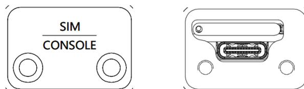
There is a secure lock panel on the right side of EG500 to protect the SIM card and Console port from external unauthorized extraction or tampering. You are allowed to install SIM card and connect USB-C console port after unlock the cover screws.
