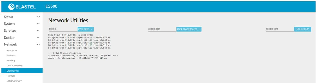
The screenshot shows the 'Network Utilities' section of the ELASTEL EG500 webUI. It features three tabs: 'IPV4 PING', 'IPV4 TRACEROUTE', and 'NSLOOKUP'. The 'IPV4 PING' tab is active, displaying the results of a ping test to 8.8.8.8. The output shows four successful ping attempts with varying response times (62.077 ms to 69.543 ms) and a summary indicating 5 packets transmitted, 5 received, and 0% packet loss.
