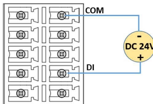
EG500 provide 6x DI to detect the status of outside digital signal, also support count mode to calculate the frequency.
