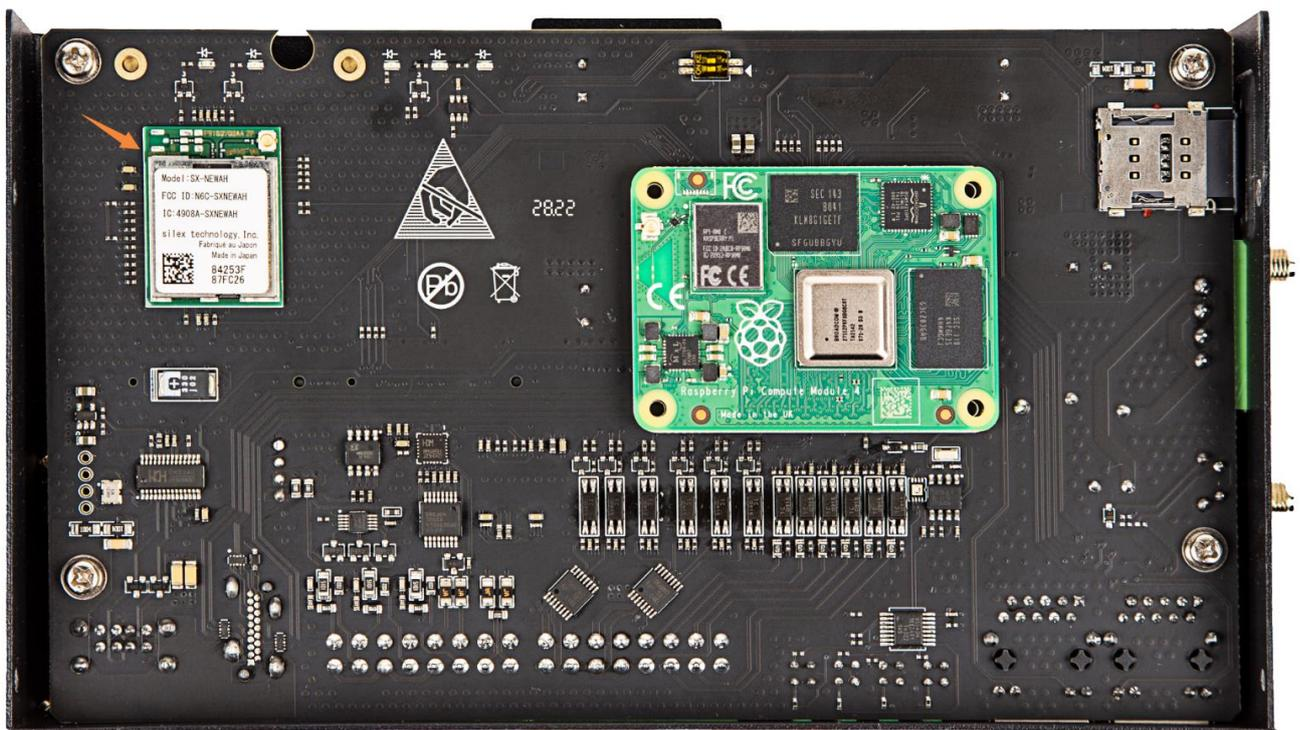
EG500 IoT gateway support 802.11ah WiFi (also named WiFi HaLow) network powered by SX-NEWAH module from SilexTechnology, the first industrial IEEE 802.11ah Wi-Fi module that operates in the **Sub 1GHz** band.
