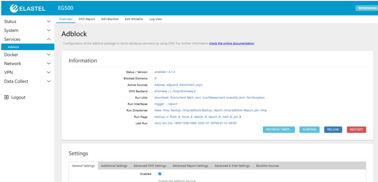
The screenshot shows the 'Adblock' service configuration page in the ELASTEL webUI. The left sidebar contains a navigation menu with options like Status, System, Services, Docker, Network, VPN, Data Collect, and Logout. The top header displays 'ELASTEL EG500' and a 'REFRESHING' button. The main content area is titled 'Adblock' and includes a sub-header 'Information' with a table of service details and a 'Settings' section with a toggle switch for 'Enabled'.
