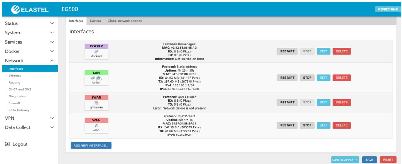
Network menu provide the network management related settings like interfaces, wireless, DHCP, LoRa Gateway.....and so on.
